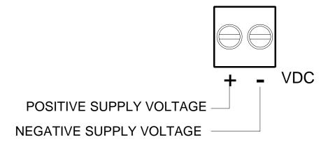
**NOTE:** The PRO DC grounds the negative power supply lead. The PRO DC can not be powered from a positive grounded system.
